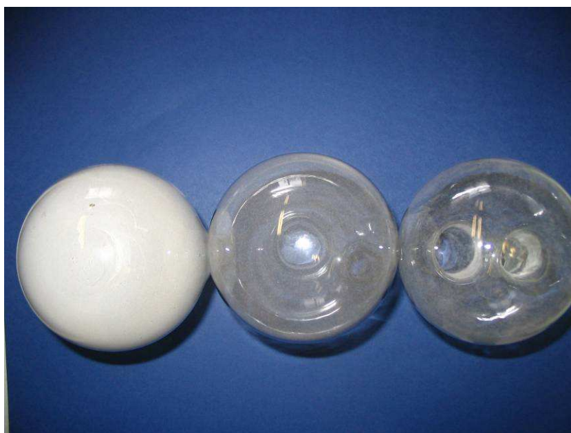
Figure 8. Flasks used for heating untreated water, water treated with home-made magnetic device and water treated with magnetic descaler Elcla
