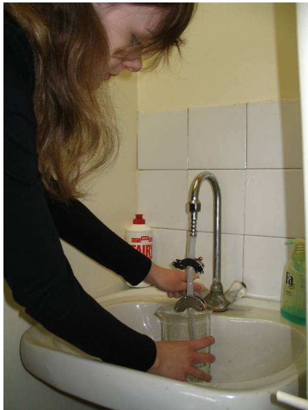
Figure 4. Water treating with home-made magnetic descaler
